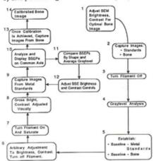
recalibration would be performed if BSEP changes of greater than 1.5 percent were observed. This work demonstrates that it is possible to calibrate SEM operating conditions (brightness and contrast) using pure materials. In addition, this scheme can be used to study mineral changes in individual trabeculae of cancellous bone, which previously had no accurate method for quantifying mineralization at a microscopic level. A real-time, automated calibration method is currently being devised.
