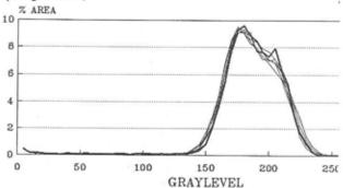
Figure 5 - BSEPs for baseline image and five calibration trials, showing the reproducibility for bone.
